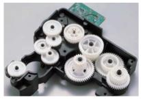
Polyacetal is used in drive gears in laser printers.
